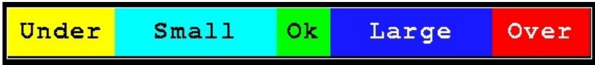
Figure 2: Graphical representation of Checkweigher zone configurations.
